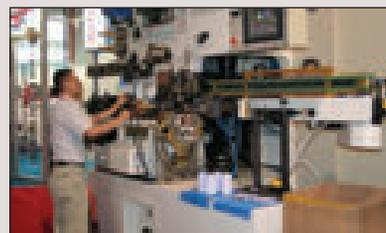
touch-screen operation, servo feeding and punching. It is also equipped with double-sheet detector, overload and double-punching protection system. The maximum output is 300 units a minute with three-out tooling.
