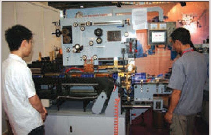
At Cannex Asia Pacific, Wantong Can-making Machinery demonstrated this welder for making round cans between one and five litres that runs at 45cpm
