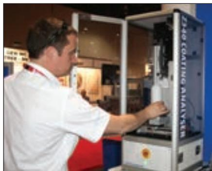
ment system for in-process measurement of wet or dry flat sheets and coils, designed to improve coating quality and reduce production costs.
